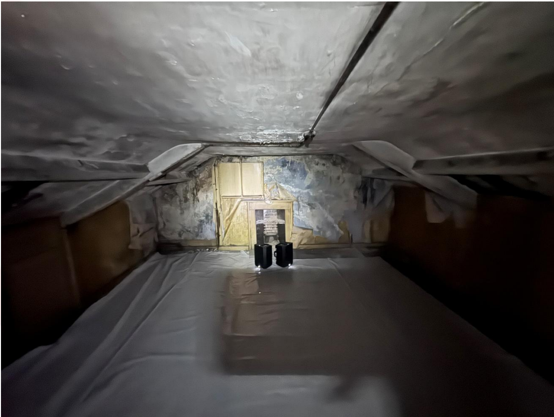
Figure 3: Noise break-out measurements in progress
